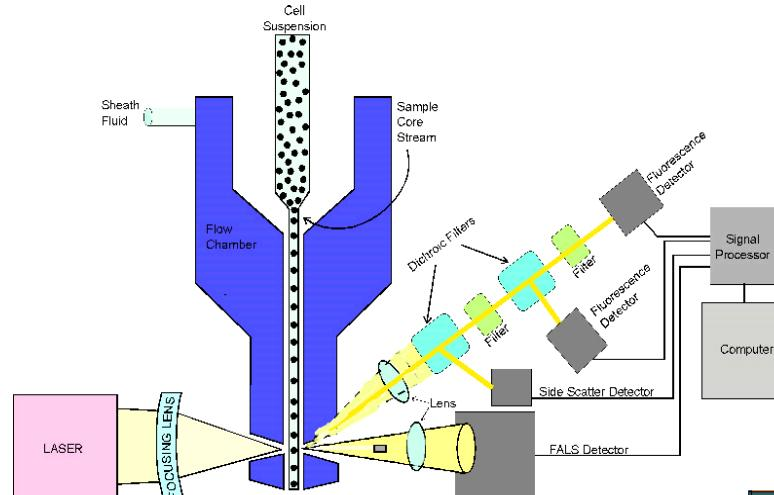
Schematic of flow cytometer instrument
